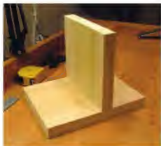
The basics. The vertical board is the tenon piece which will be joined to the face of the mortise piece.
